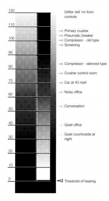
Figure 1 Some typical dB(A) noise levels
