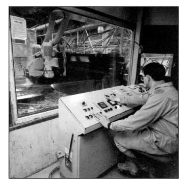
Figure 9 Remote/automatic control of saws
