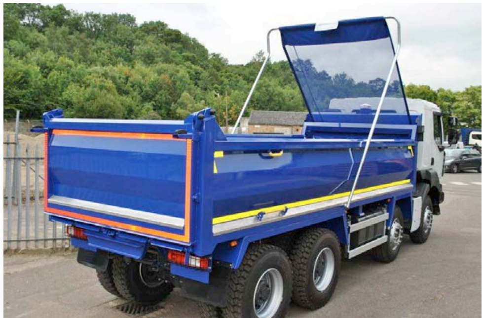
Figure 20 Front-to-rear sheeting system
