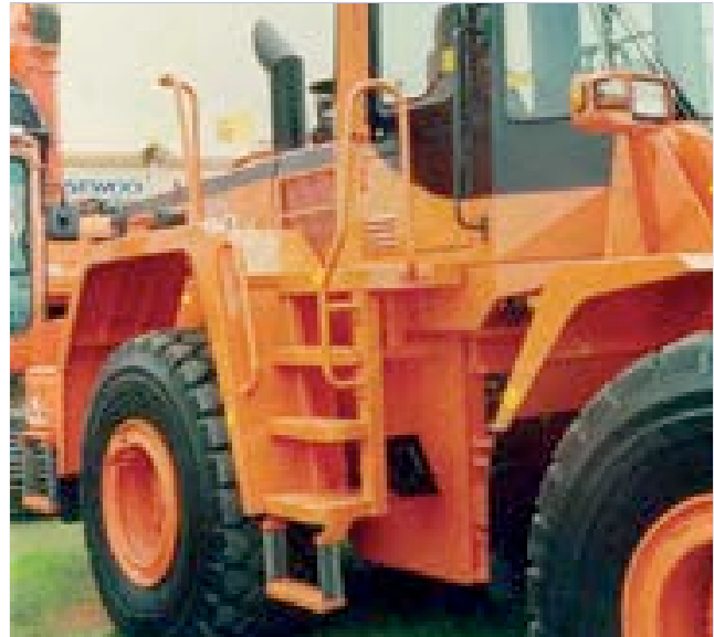
Figure 18 Access to vehicles – steps and handrails
