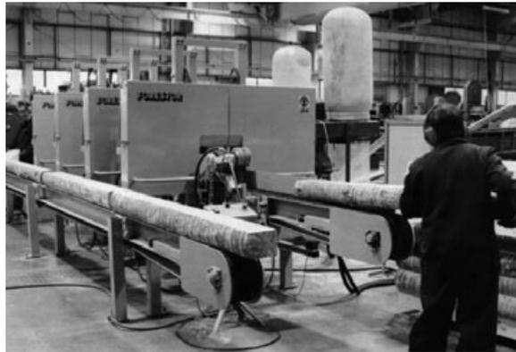
**Figure 4b** Hand-fed multi-cut band re-saws
