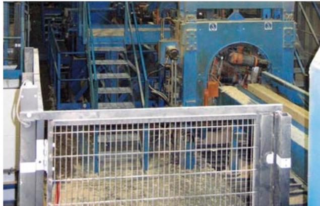
**Figure 26** Auto log processing + safety barrier
