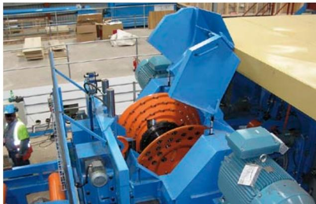
**Figure 27** Chipper/reducer and covers
