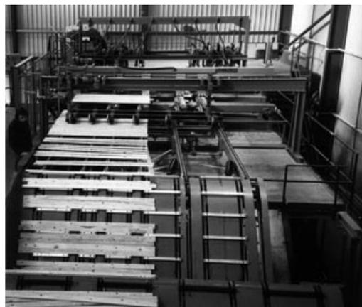
**Figure 23** Automatic stacking machine
