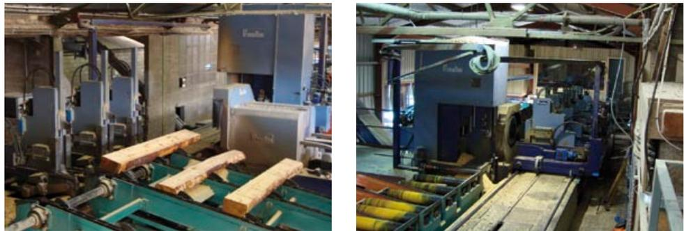
**Figure 8** A reciprocating carriage log band saw – feed on to carriage and carriage approach to band saw
