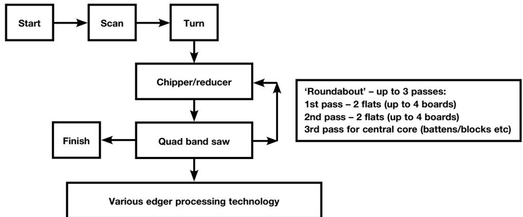
Figure 29 A typical mechanised sawmilling line
