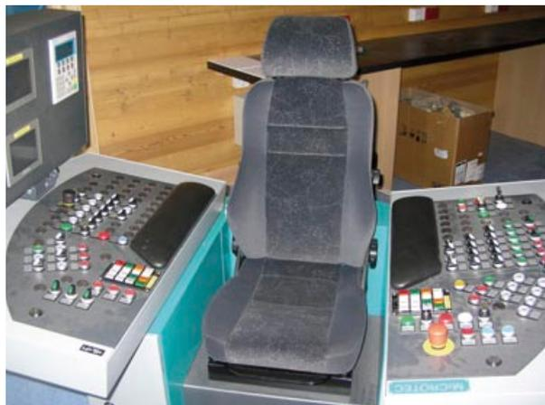
**Figure 31** Automated sawmill control room
