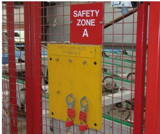
**Figure 30** Safety lockout station
