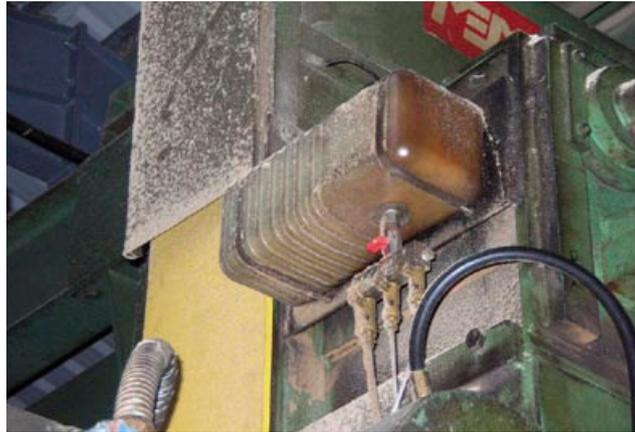
**Figure 2** Automatic lubrication system
