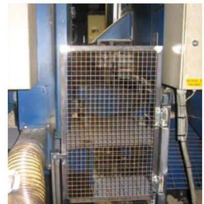
**Figure 6** Older mechanically-fed six-in-line horizontal band saws with retrofitted interlocked hinged gate between machines
