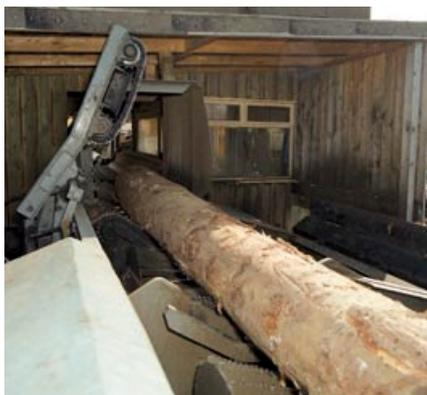
Figure 24 Butt reducer
