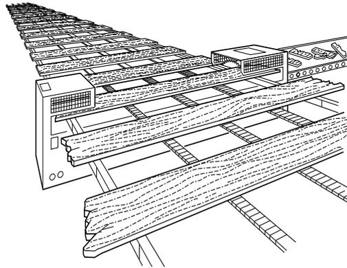
**Figure 19** Trim saws fed by chain conveyors
