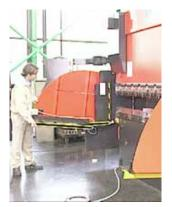
Light curtain which can have its assembly rotated to alter the angle of approach
