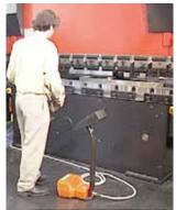
Combined vertical and horizontal light curtain applied to a hydraulic press brake
