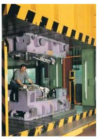
Hydraulic press, Type 4 external ESPE with internal laser scanner
