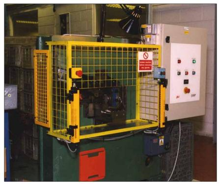
Test rig with combination of protective measures including light curtain
