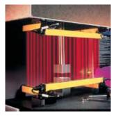
Minimum separation distance must be calculated to allow safe application of the light curtain
