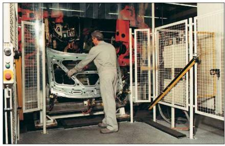
Robot load bay with Type 4 ESPE
