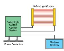
ESPE interfacing with the machine control system providing monitoring of the light curtain and power contactors
