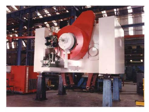
Clutch-brake unit for large power press
