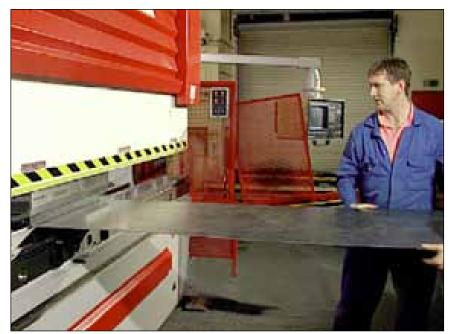
Hydraulic press brake with horizontal light curtain
