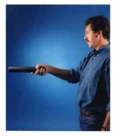
Insert the appropriate diameter test piece into the light curtain
