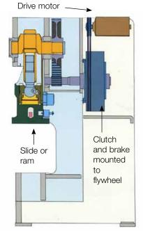
Cross section of a typical power press
