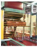
Stretch wrapper with lifting table (light curtain protected by IP67 polycarbonate tubes)
