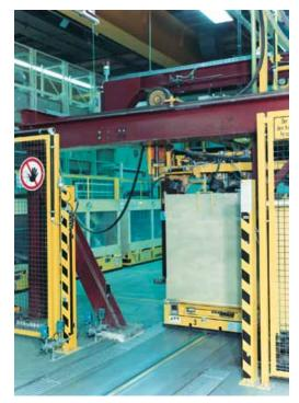
Entry-exit system. Four beam muting, three beam guard
