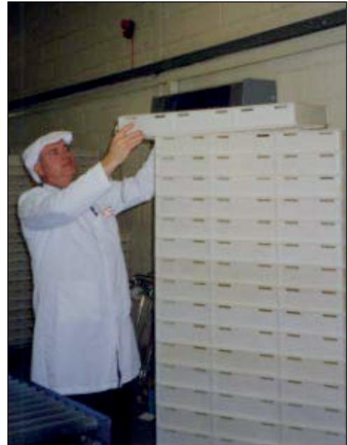
The weight of each tray was between 5 and 10 kg, and the dimensions of each tray were 75 x 40 x 10 cm. The total weight of a stack of trays could be as much as 200 kg. Trays were often overloaded, and/or asymmetrically loaded so they were heavier at one end than the other. There were no (designed) hand holds on the trays, although the sides were relatively easy to grip. The total height of a stack of 20 trays and a trolley was 215 cm.
