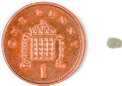
Figure 3 Comparison of an accumulation of RCS dust with a penny
