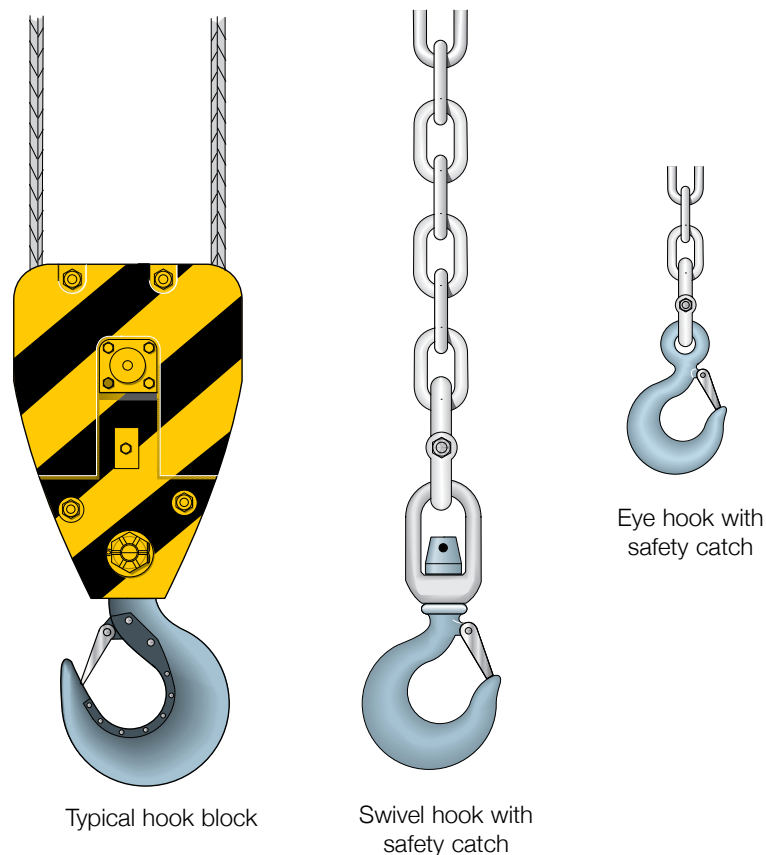
Figure 4 Some types of hooks found on cranes and lifting equipment
