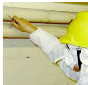
Figure 9 Taking a sample with a corer for a Type 2/3 survey
