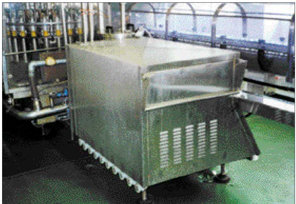
Solution: acoustic hood fitted over filler pump
