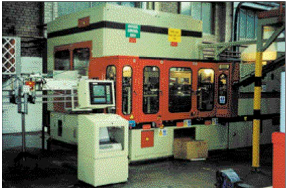
Problem: bottle-blowing machine in production hall before being relocated in separate room
