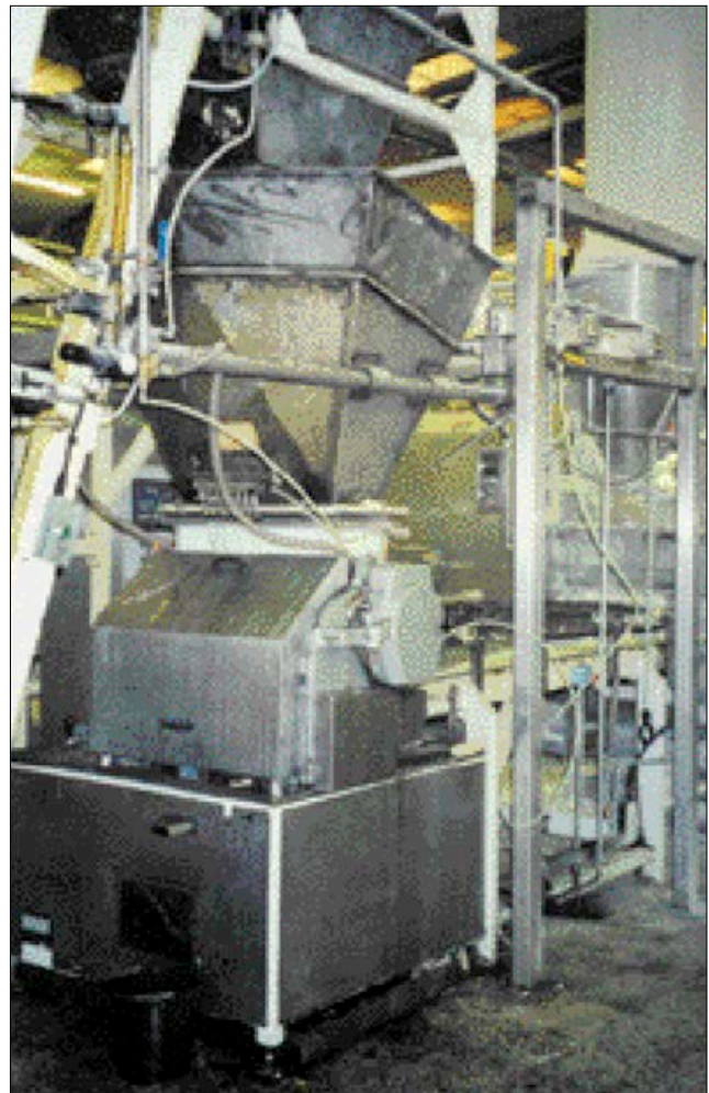
Solution: mechanical modifications on dough mixer halved noise level
