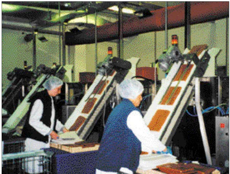
Solution: plastic chutes for toffee transfer
