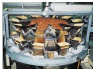
Solution: hoppers internally coated with damping material
