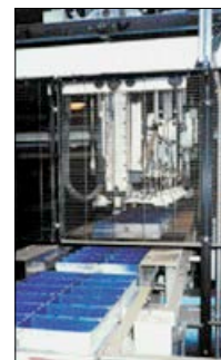
Solution: new robot installed to change tins
