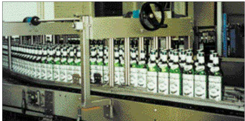
Solution: new variable-speed conveyor with adjustable guide-rails
