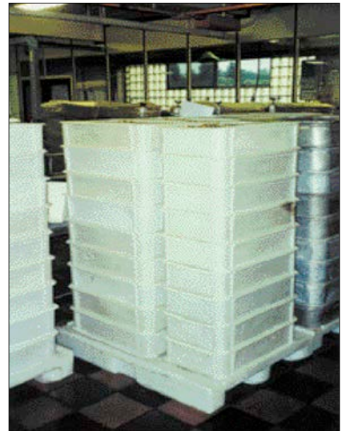
Solution: plastic trays now used to reduce noise
