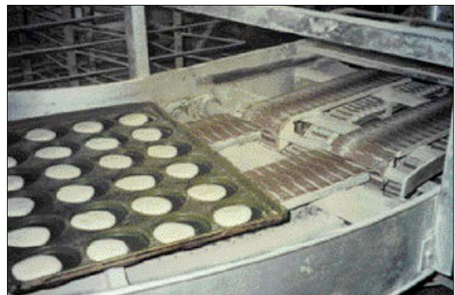
Solution: new plastic tracking on conveyor
