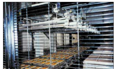
Solution: new robot installed for lidding/de-lidding tins
