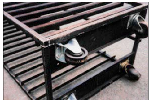
Solution: rack with new phenolic wheels
