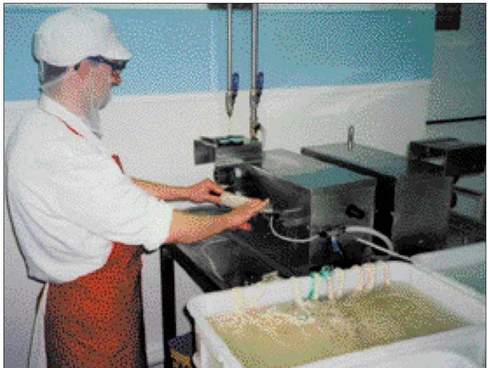
Solution: new, quieter compressed-air spooler
