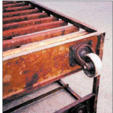
Problem: rack fitted with original metal wheels
