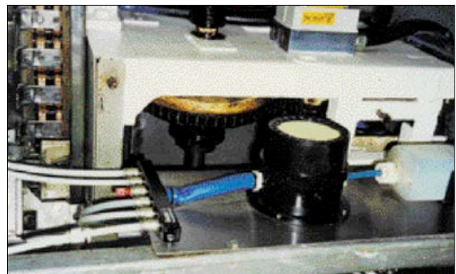
Solution: new, quieter water pump
