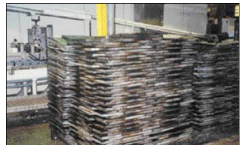
Problem: storage of lids for manual lidding
