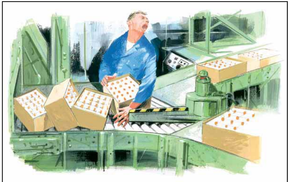
Figure 5 Operator traps hand in automated transit system
