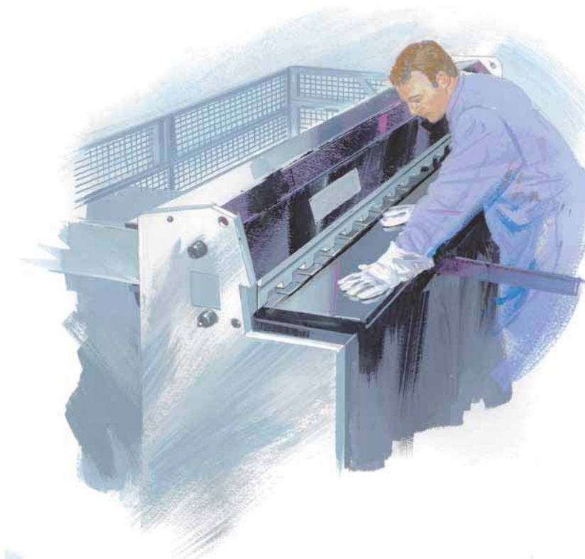
Figure 9 Use of a hydraulically operated guillotine
