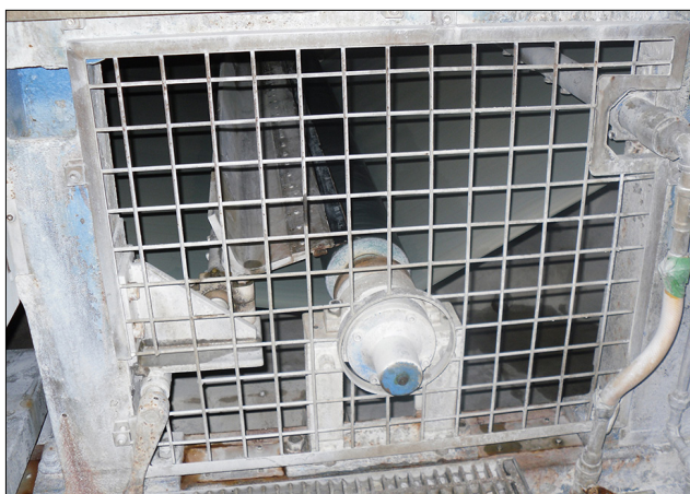
Figure 27 Fixed guards to prevent access to moving rolls underneath the wire
