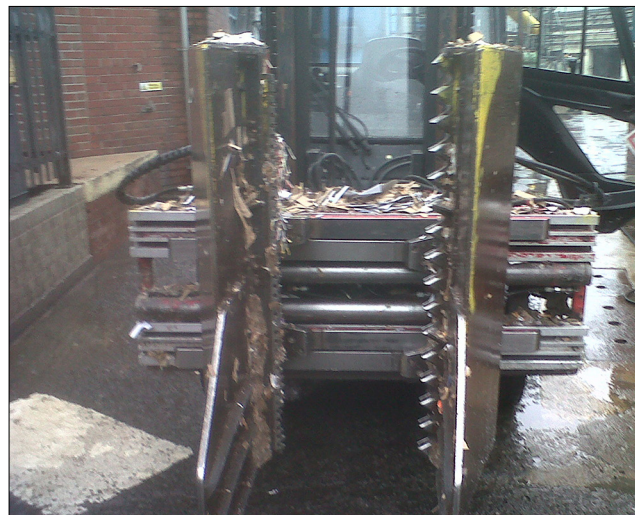
Figure 15 An example of a forklift truck with serrated clamp arms to cut bale wire
