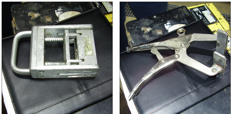
Figure 12 Examples of devices that could be used to pull the felt into position.
