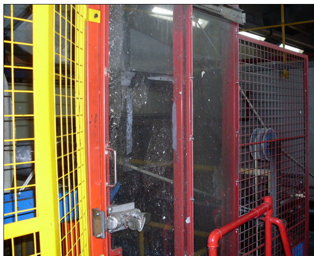
Figure 3 Example of a movable guard
