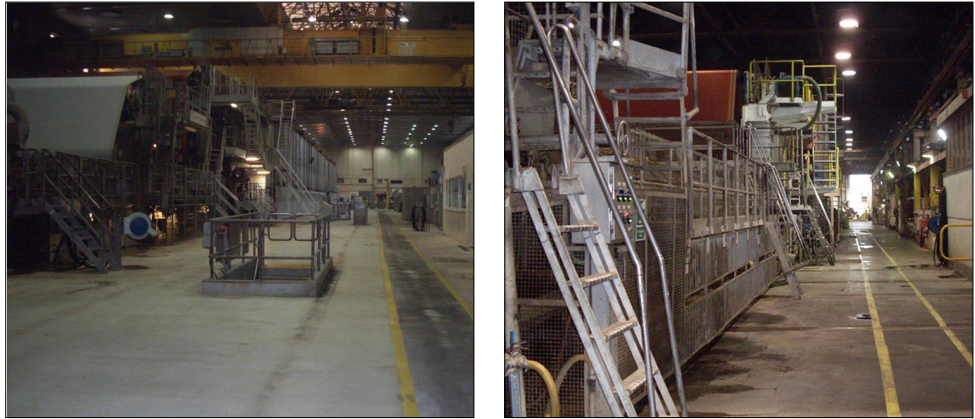
Figure 11 Areas around the paper machine, including the basement, should be kept clear at all times
