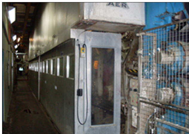
Figure 29 Interlocked hood doors can be used to prevent access to the drying cylinders
