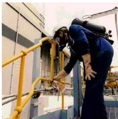
Testing for leaks with ammonia bottle (see also para 208c). The driver tests the joints near the tanker dome
